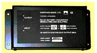
**GENERAL DESCRIPTION.** A small converter, generating a range of standard voltages, capable of powering most battery equipment when supplied from 60, 72V or 84V batteries. The input and output are ohmically isolated, making installation very simple. The output has a constant current limit.
