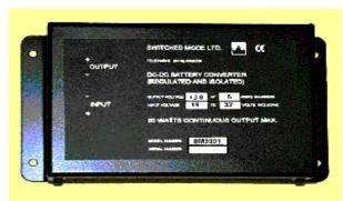
**GENERAL DESCRIPTION.** A small converter producing up to 120W (478X series) or 200W (479X series) with a range of dc outputs, when supplied from a 24 or 48V battery. The input and output are ohmically isolated, making installation very simple. The output has a constant current limit and the unit incorporates an electronic relay to turn it on/off remotely, via a control input.
