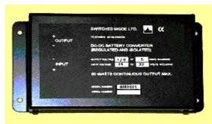
**GENERAL DESCRIPTION.** A small converter producing up to 120W (332X series) or 200W (333X series) with a range of dc outputs, when supplied from a 12 or 24V battery. The input and output are ohmically isolated, making installation very simple. The output has a constant current limit and the unit can be turned it on/off remotely, via a control input.
