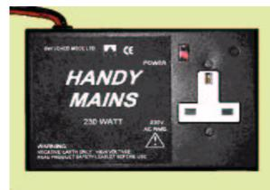
**GENERAL.** These economic power adaptors convert battery voltage to mains level voltage, for powering computers, printers, etc. The units have an output power of 250 watts short term, with surge handling up to 500 watts. Continuous available power, quoted as 200W, is limited automatically by case temperature.
